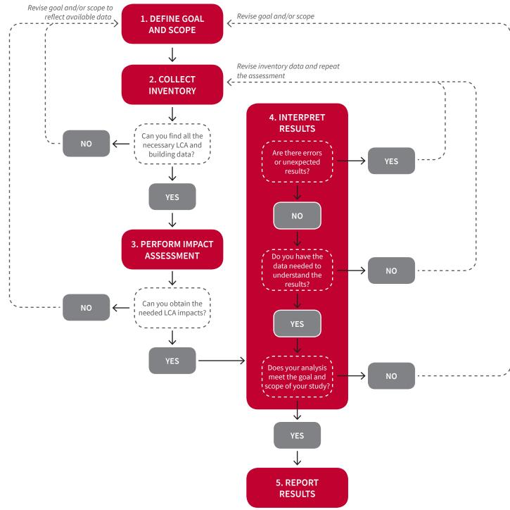
**Figure 5**. Iteration checkpoints in LCA.
