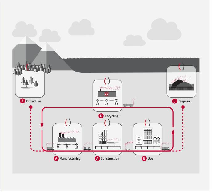
**Figure 1**. Sources of emissions by life cycle stage (A, B, C, D) of a building based on stage definitions from European Standard (EN) 15978 (credit: Meghan Lewis).
